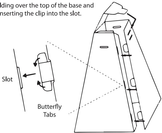
**Step 2:** Fold all creases for top unit. Assemble top by folding butterfly tabs in and inserting into the slots. Finish off the top unit by folding over the top and inserting the clip into the slot.
